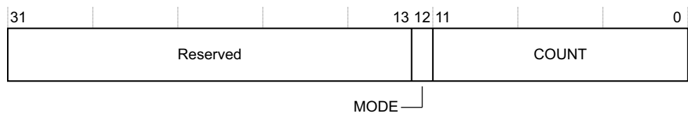
Figure 2-13 STMSYNCR bit assignments
